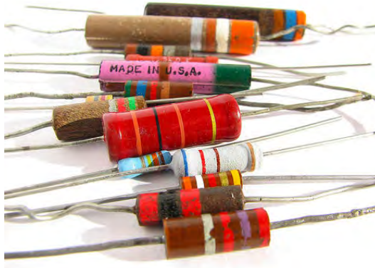
Different types of resistors used to add resistance to an electric circuit.
