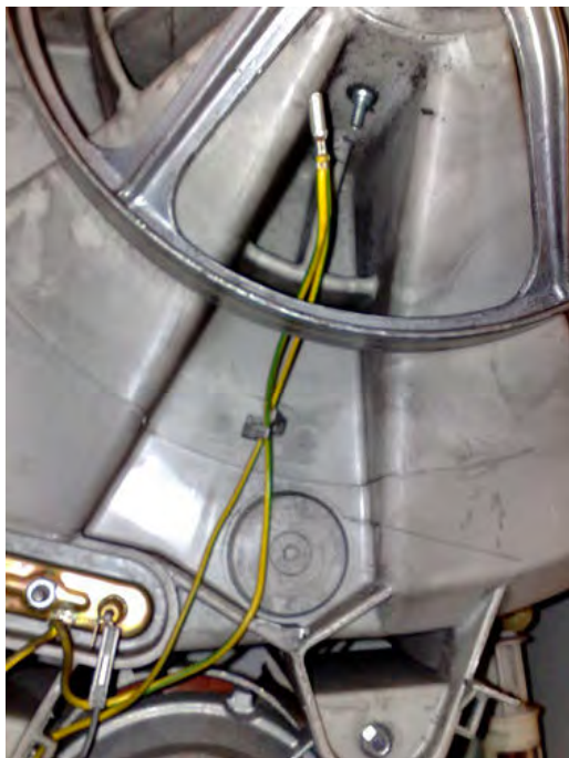
The green and yellow earth wire connected to the metal casing inside an electric motor.
