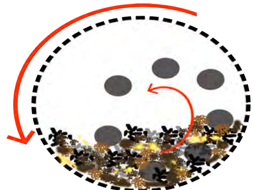
Inside a ball mill, the balls move round in a circle as the mill turns, crushing the ore into a powder.
